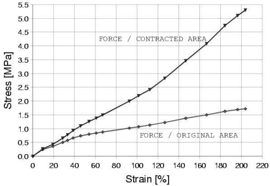
Figure 4: Stress - strain diagram of silicone rubber
