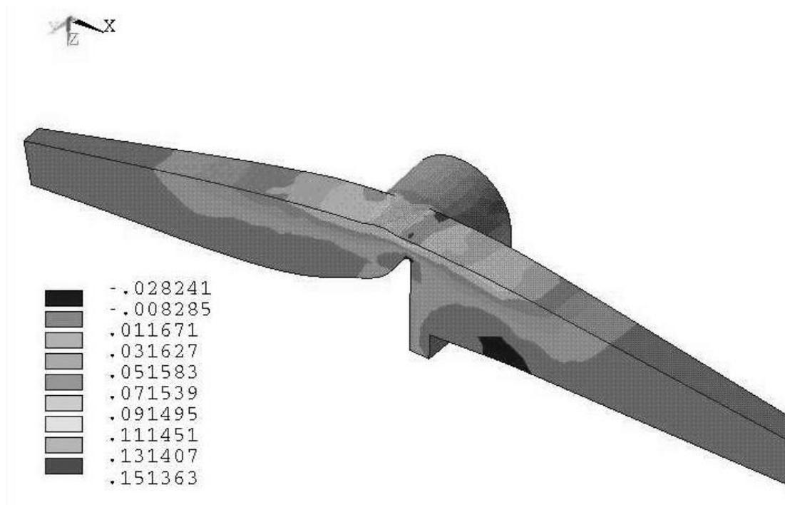
Figure 6: Stress field  $\sigma_1$  for flexion  $75^\circ$  [MPa]
