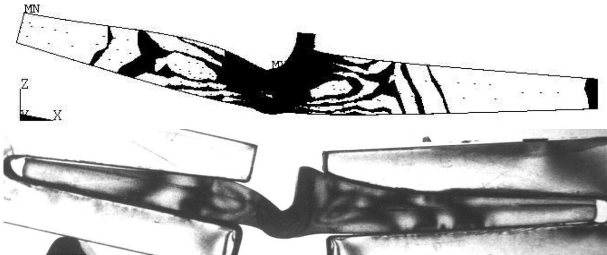
Figure 5: Comparison of principal stresses differences obtained from FEM and photoelastic model for flexion 15°
