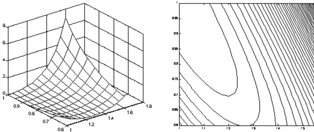
**Figure 4.** Strain energy function and its contour lines in the experimental range
