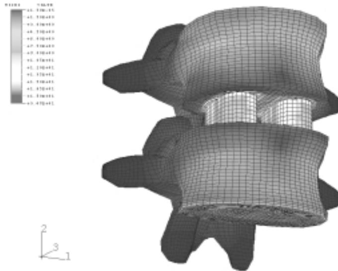
Figure 1: Von Mises stress distribution of a contact model of vertebrae L<sub>3</sub>-L<sub>4</sub> with a pair of C/C-composite implants being vertically loaded.
