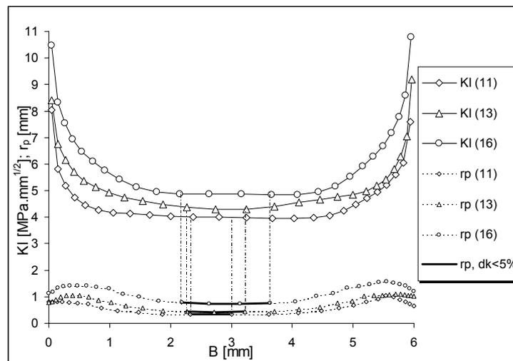
Fig.4 – Stress intensity factor and range of plastic zone in front of the real crack tips. Thick curves delimit area where is range of plastic zone increasing up to 5% of total range.
