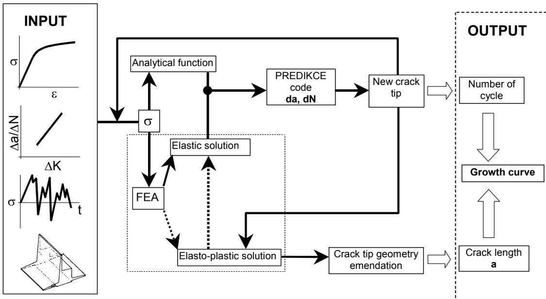
Fig.6 – Schematic technique of fatigue crack growth prediction in 3D body.
