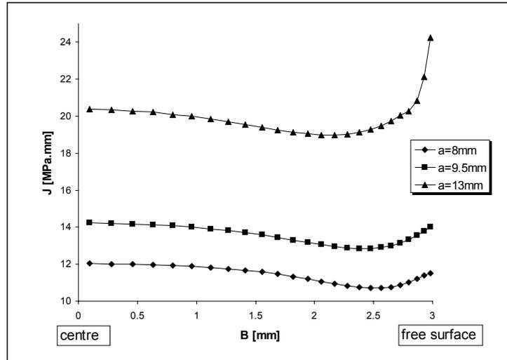
Fig.5 - J-integral value along straight crack tip for loading of maximal stress.
