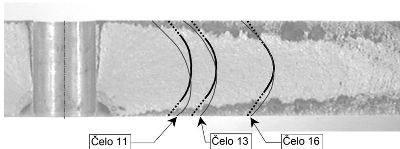
Fig.6 – Comparison between emendation straight crack tip geometry (thick curve) and real crack tip geometry (thin curve). Dotted line marked linear extrapolation of crack tip emendation towards free surface.
