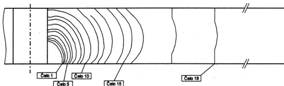
Fig.2 - The geometry of fatigue crack tips from fractographic analyses [4].
