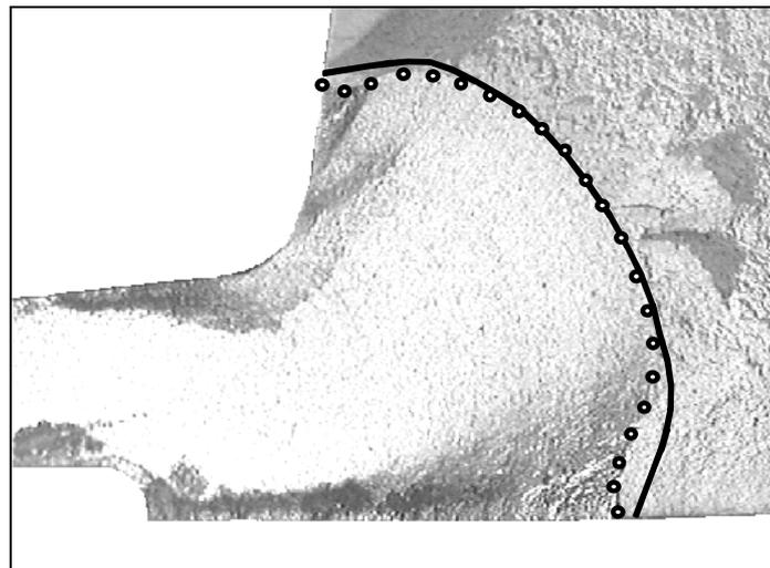
Fig.8 – Comparison between final calculation crack tip geometry (thick curve) and final crack tip geometry from experimental measurements (points).
