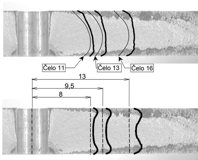
Fig.3 – The range of plastic zone (distance between thin line and thick line) in front of the real crack tip geometry (above) and straight crack tip (below).
