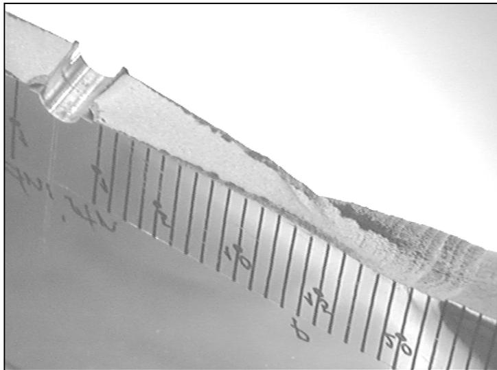
Fig.1 – Typical fracture surface on the M(T) specimen [3].
