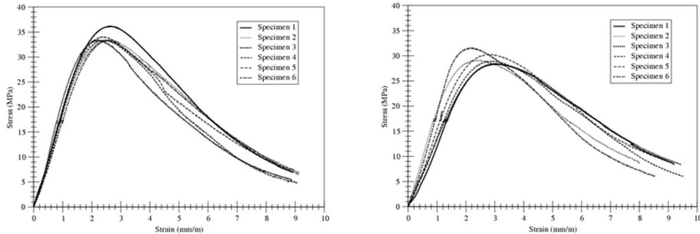
3. Stress-strain diagrams of specimens at temperature +20°C (left) and +60°C (right).
