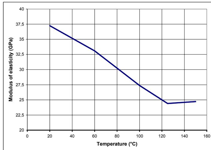
6. Relation between modulus of elasticity and temperature.
