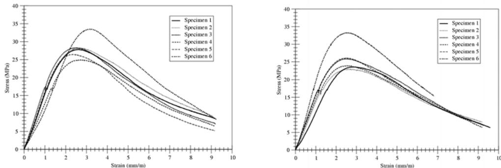
4. Stress-strain diagrams of specimens at temperature +100°C (left) and +125°C (right).
