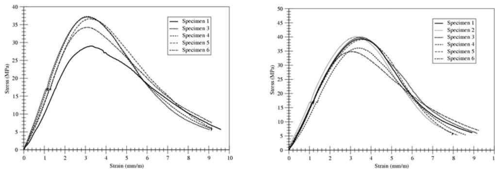
5. Stress-strain diagrams of specimens at temperature +150°C (left) and +200°C (right).
