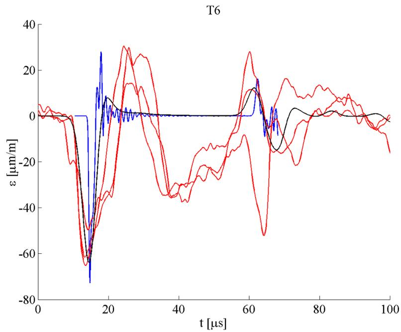
Figure 3: Measured and calculated time history of strain in T6 strain-gauge (red – measured, blue – contact FEA, black – point-load FEA).
