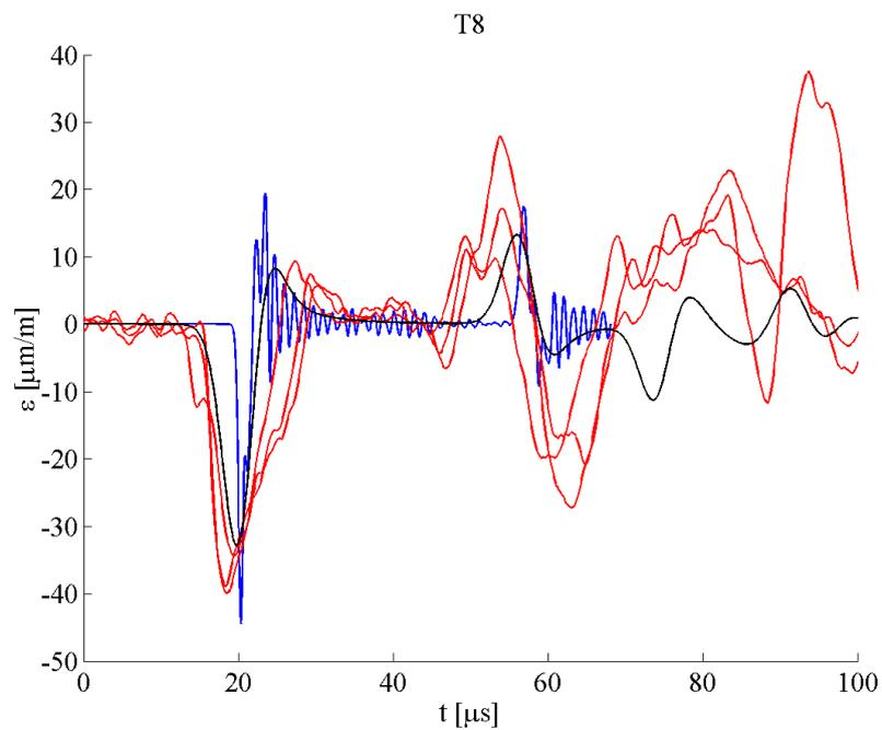
Figure 4: Measured and calculated time history of strain in T8 strain-gauge (red – measured, blue – contact FEA, black – point-load FEA).
