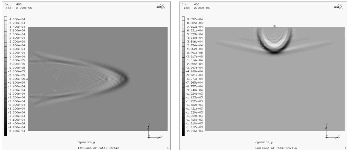
Figure 5: Contours of strain after the impact of projectile.
