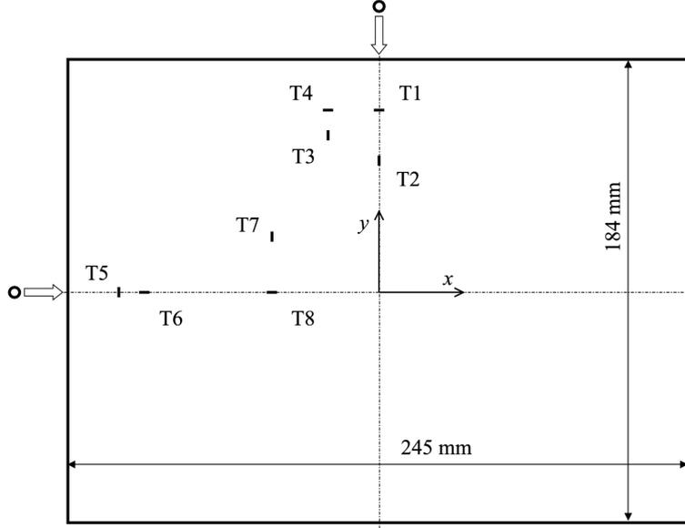
Figure 1: Geometry of the panel, strain-gauges layout and the impact fashion.
