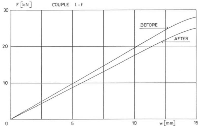
Fig. 4 Comparison of results obtained before and after dynamic test
