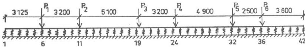
Fig. 3 Computing model of a rail
