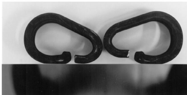
Fig. 5 Overloaded tension clam
