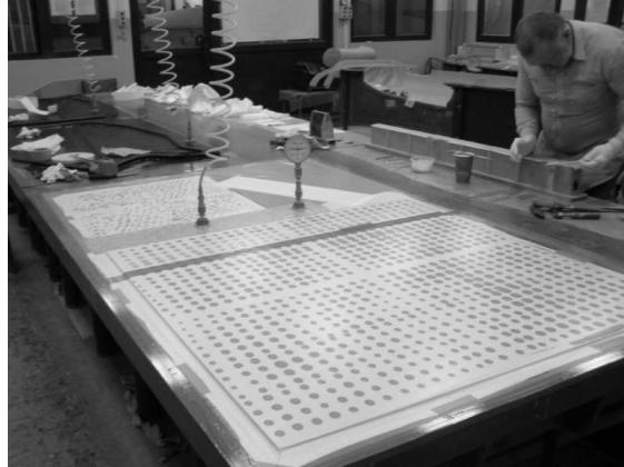
Fig.4 Sandwich semi-finished product final preparation in the workshop
