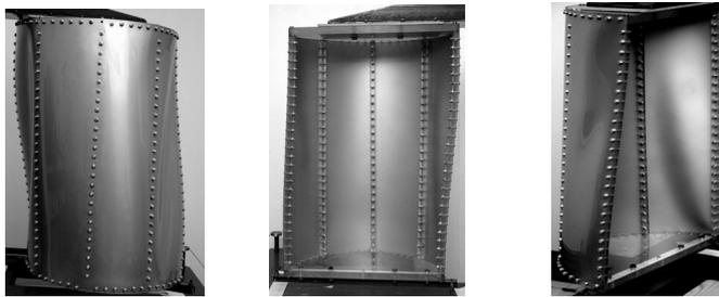
Fig.11 The structure reinforced with five stringers. Early phase of post-buckling elastic deformation.  $M_t=35$  Nm
