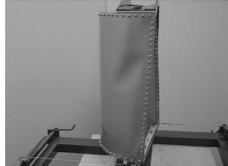
Fig.7 Beginning of local buckling.  $M_t=25$  Nm
