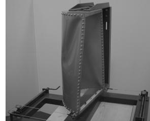
Fig.8 The next phase of post-buckling state.  $M_t=35$  Nm
