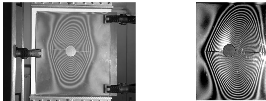
Fig.5 Moiré fringes illustration Quantitative of deflections in proximity of the crack
