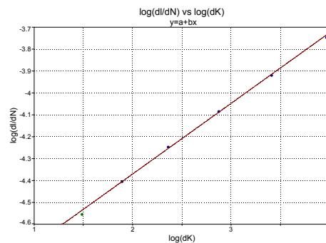
Fig.7 Dependence  $\log \frac{da}{dN}$  versus  $\Delta K$
