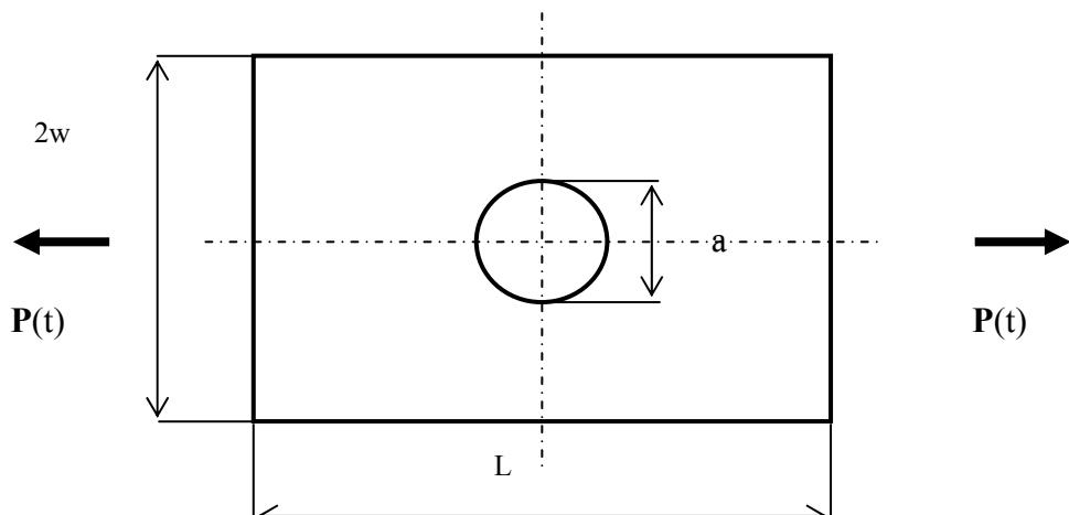
Fig.2 Dimensions, circular hole location and loading of the plat
