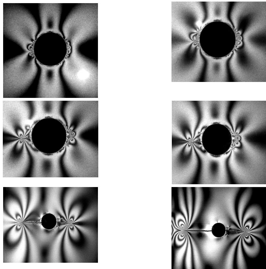
Fig.4 Field of isochromatics in the successive stages of propagation process.
