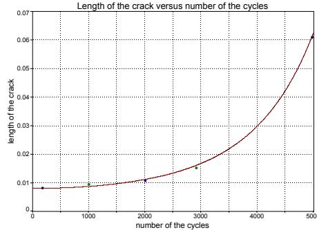
Fig.6 Dependence length of the crack vs number of cycles
