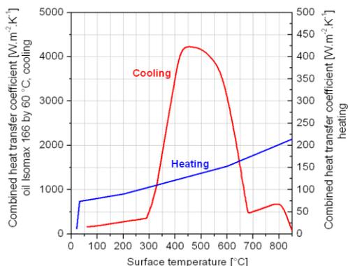
Fig. 2 Combined heat transfer coefficients
