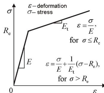
Fig. 4 Elastic-plastic material model
