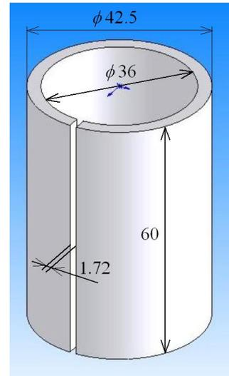
Fig. 5 Dimensions of sample
