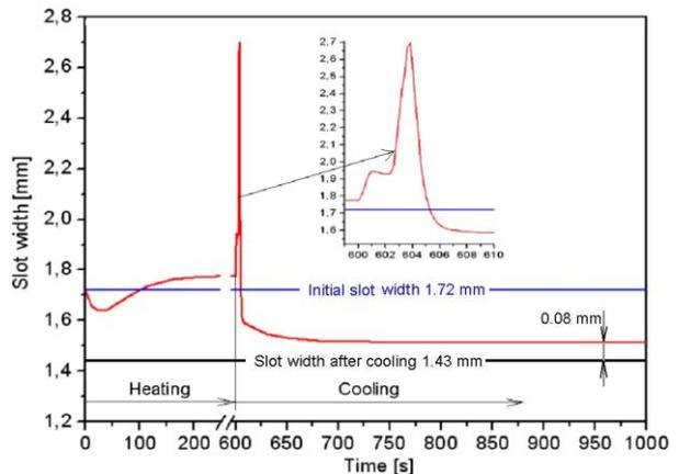
**Fig. 9** Slot width time dependence
