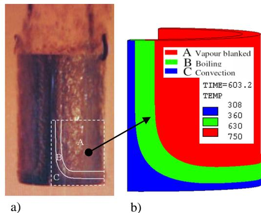
Fig.7 Temperature field [°C], cooling time 3.2 s, a) photo, b) numerical simulation
