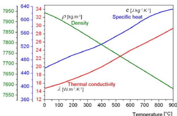
Fig. 1 Thermophysical material properties
