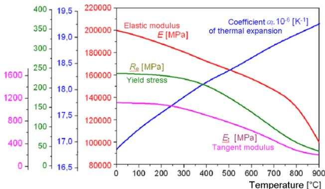
Fig. 3 Thermomechanical material properties
