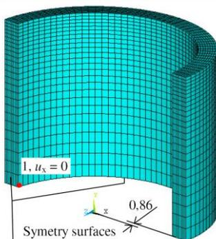
Fig. 6 Geometrical model with generated mesh
