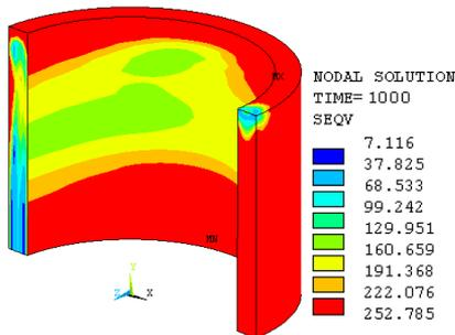
**Fig. 8** Residual equivalent von Mises stress field [MPa]
