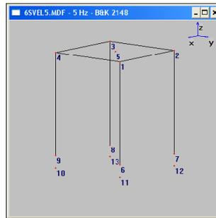
**Fig. 2** The point grid for modal shape measurement
