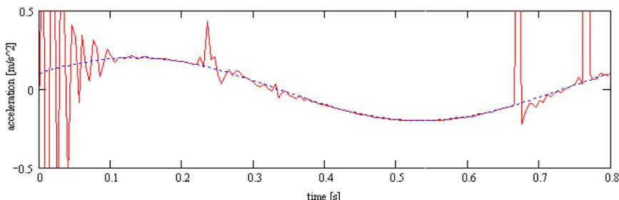
**Fig. 3** Comparison of assumed and MSC.ADAMS simulated acceleration course.
