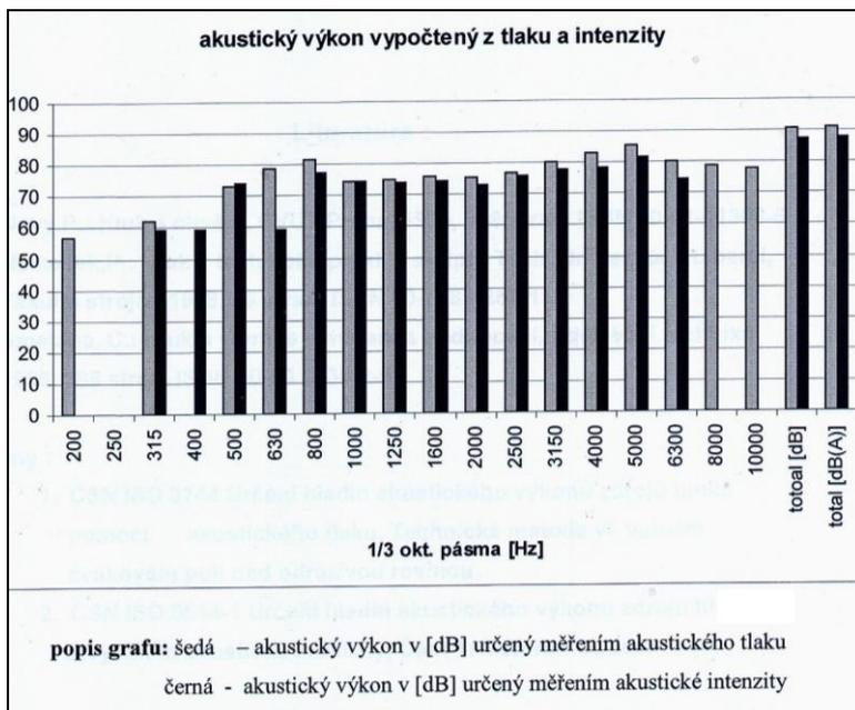
**Fig. 1** Comparison of acoustic pressure and acoustic intensity measurements
