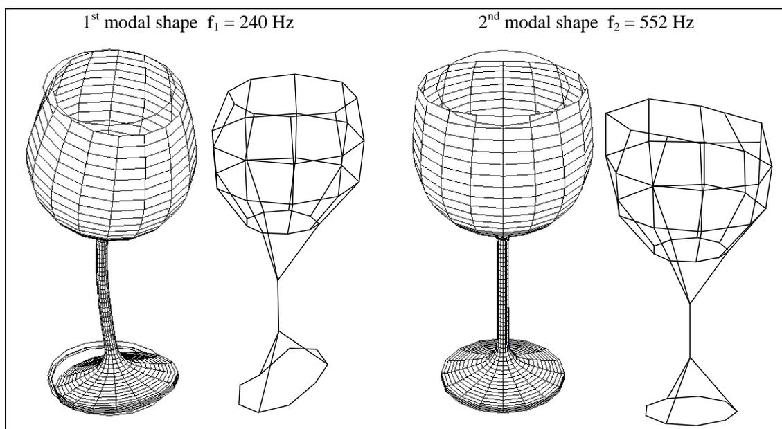
**Fig. 1** Comparison of computational and experimental modal shapes
