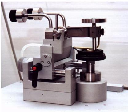
Fig. 4 Tribometer ball-on-disc
