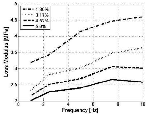
Fig. 3 Storage and loss modulus for different strain amplitudes - material B
