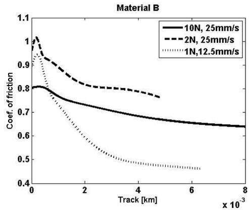
**Fig. 7** Friction coefficient material B
