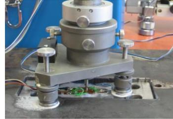
**Fig. 4** Positioning of specimen into frame
