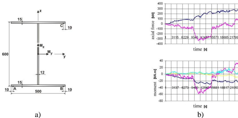
**Fig. 7** Time dependent charts of axial forces and bending moment increments in columns cross-sections during boiler operation
