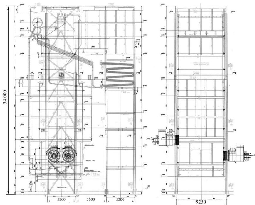
**Fig. 3** Steam boiler with basic dimensions of supporting structure
