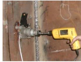
**Fig. 5** Drilling in strain gage rosette by RS-200
