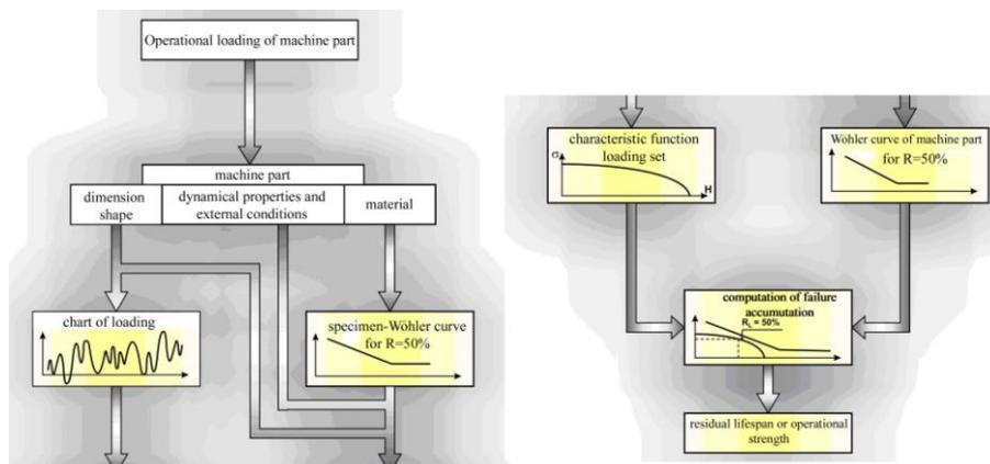
**Fig. 8** Assessment of lifespan or residual lifespan
