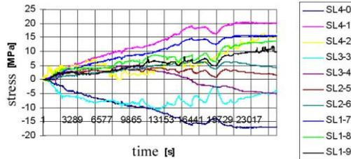
**Fig. 6** Charts of time dependent stress increments in columns of supporting structure during boiler operation
