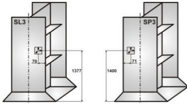
**Fig. 4** Locations for application of strain gages for residual stress measurement
