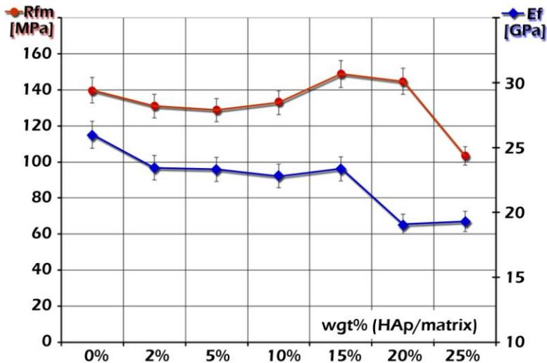
**Fig. 2** Ultimate strength in bending *Rfm* and modulus of elasticity in bending *Ef* of composites with HAp nanoparticles
