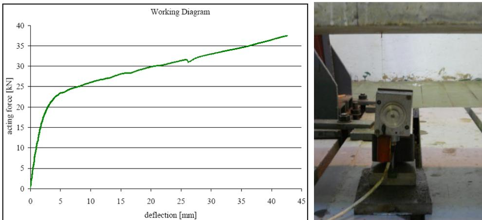
**Fig. 2** Bi-linear working diagram and deflectometer
