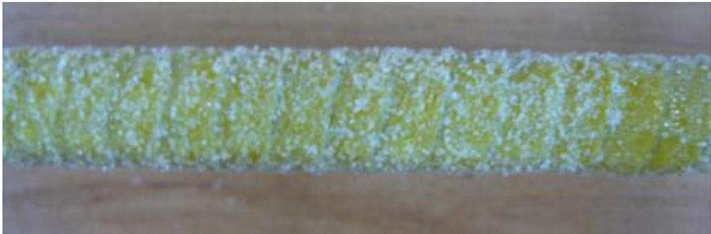
Fig. 7 Detail of the GFRP $\phi$ 14 bar
