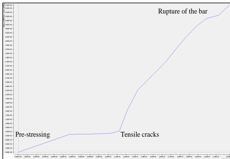
Fig. 8 Stress development in the GFRP $\phi$ 14 bar
