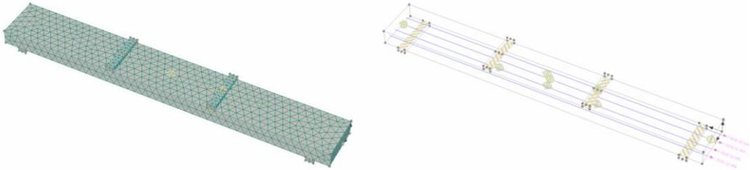
**Fig. 4** ATENA model – mesh and pre-tensioning
