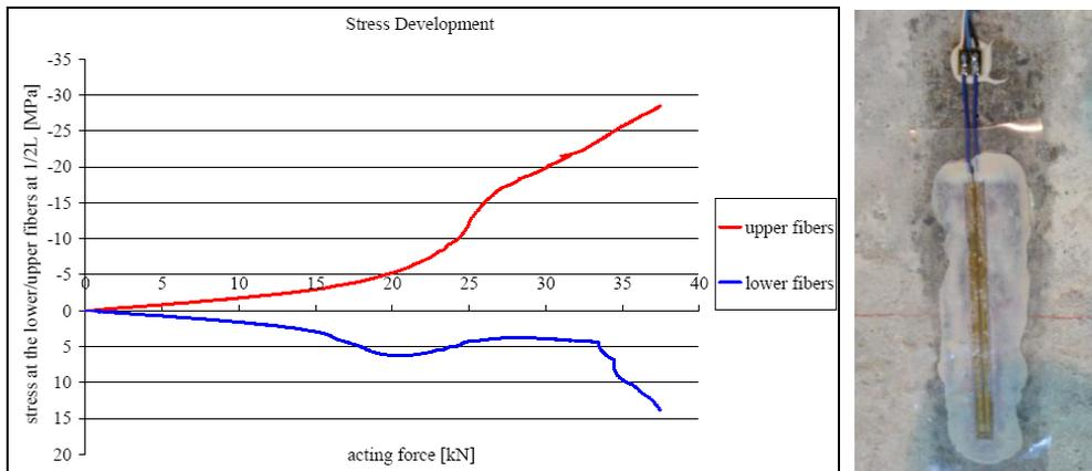
**Fig. 3** Stress development and strain gauge
