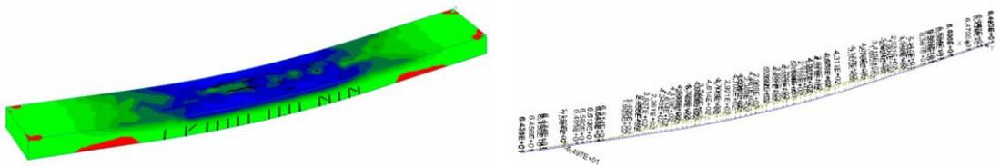
**Fig. 6** Stress in the concrete and in the GFRP bar
