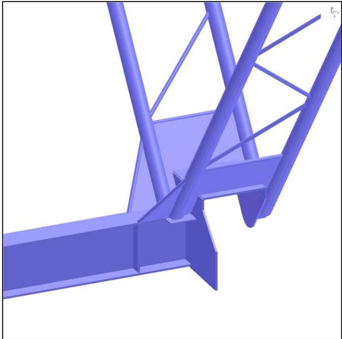
**Fig. 3** Frame cornet 3D model – shell elements
