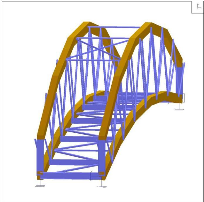
**Fig. 2** Front view of the footbridge
