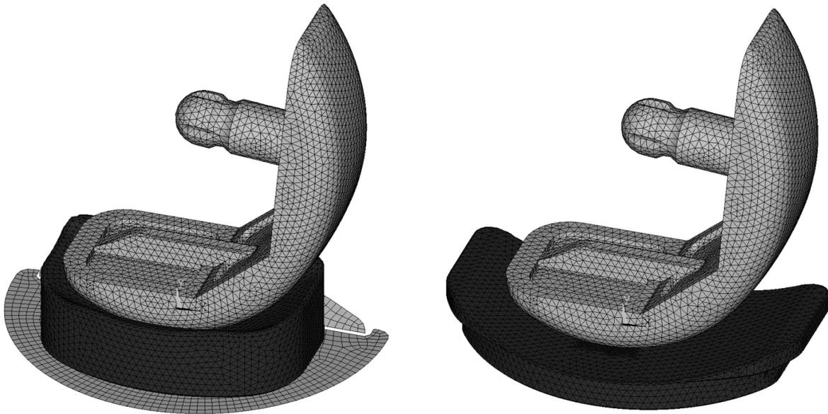
*Figure 5: Meshed models of both unicondylar knee replacements types*
