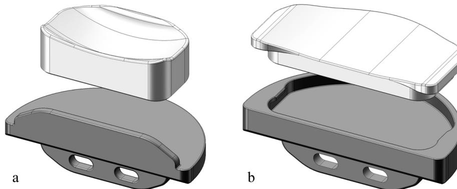
**Figure 2:** Two constructional options of partial knee replacement a) free PE housing b) fixed PE housing
