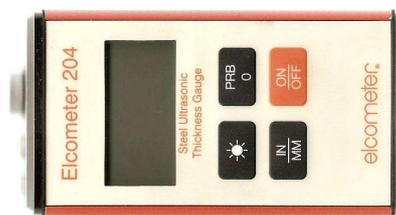
**Figure 5:** The ultra-sound thickness-gauge ELCOMETER
