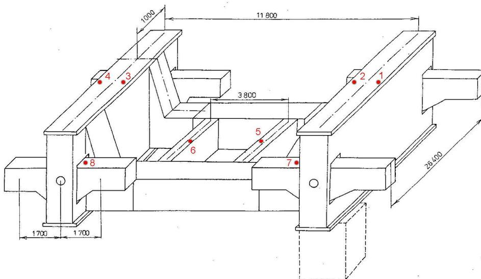
**Figure 1:** Scheme of the foundry crane 250t /63t/12,5t – 26,4 m with marked points of strain gauge arrangement
