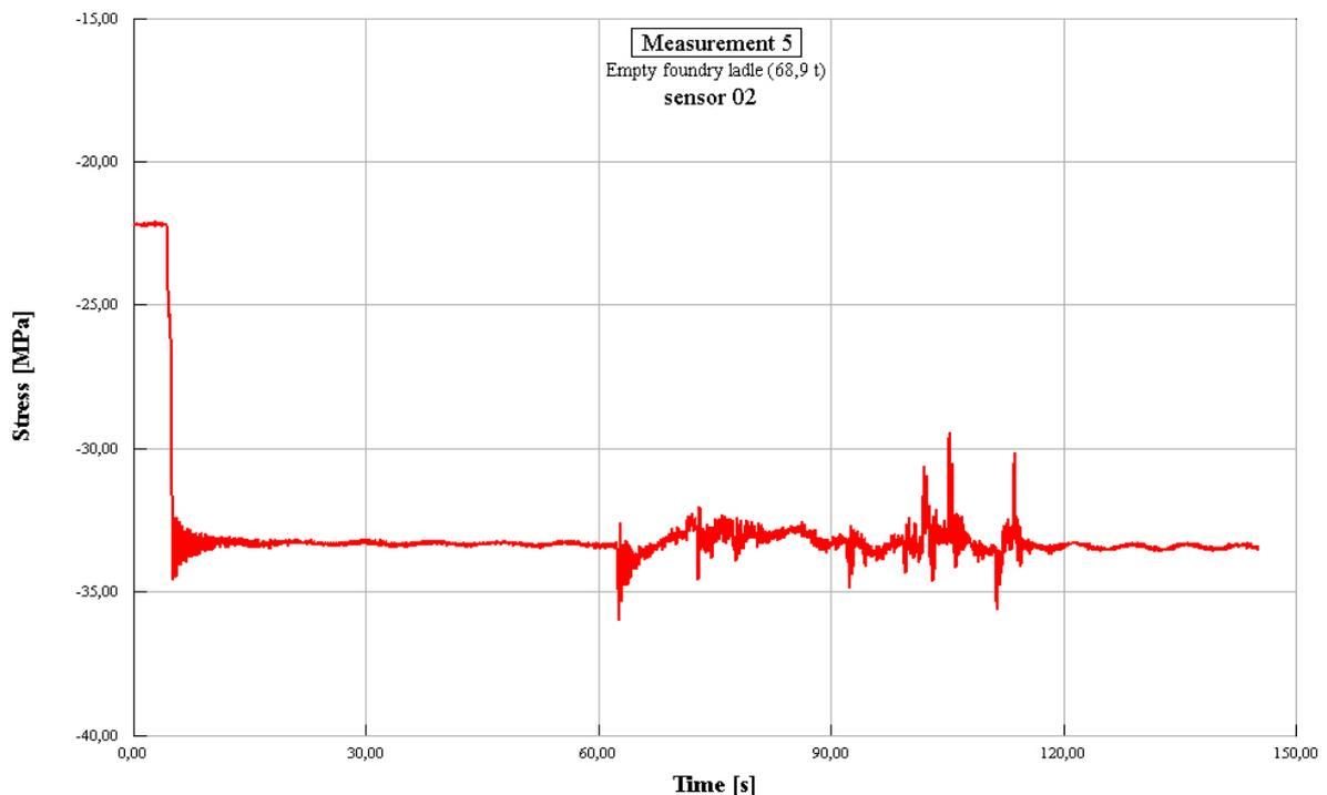
**Figure 8:** Time behaviour of loading for determination of dynamic hoisting coefficient
