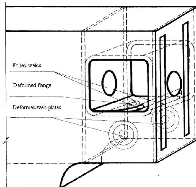
*Figure 3: Damage of main girder, illustrated schematically*
