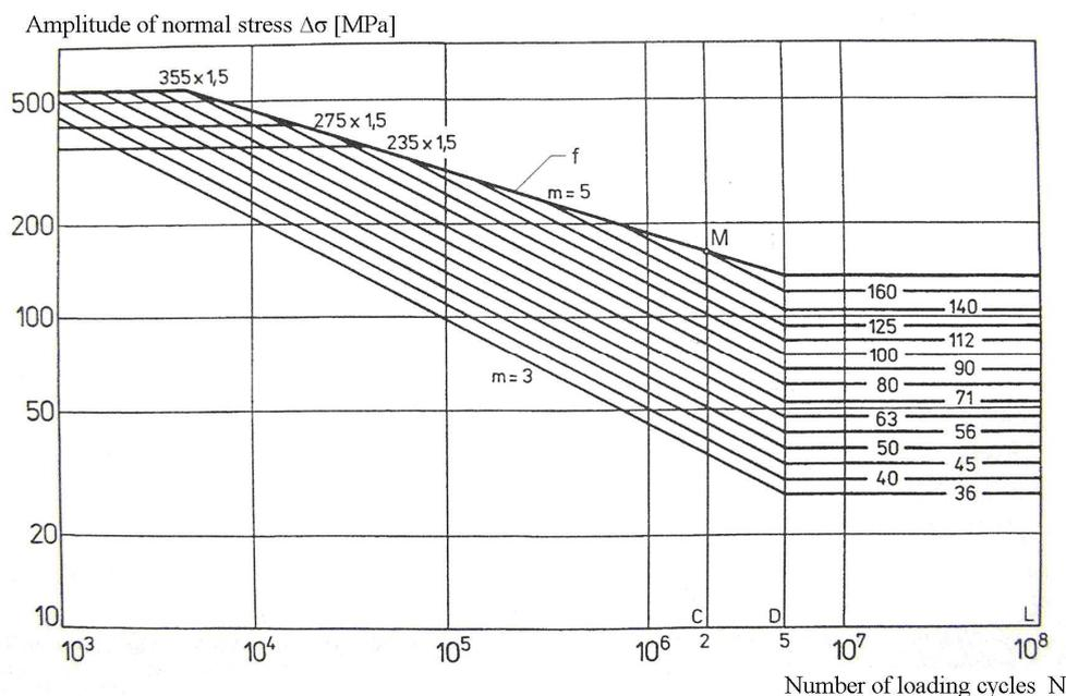
**Figure 10:** Dependence between amplitude of normal stress  $\Delta\sigma$  and number of loading cycles  $N$  for various categories of details
