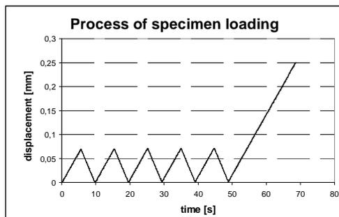
**Figure 1:** Time-displacement loading curve of randomly chosen specimen.
