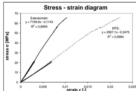
**Figure 2:** Difference of stress-strain curves obtained by MTS and extensometer.
