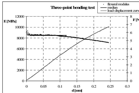
**Figure 4:** The time-history of randomly chosen specimen (Filtek™ Silorane). Dots represent calculated instantaneous values of flexural modulus. Thick line is the median of flexural modulus values in the linear region of the load-displacement curve. Thin line represents load-displacement curve of the test.
