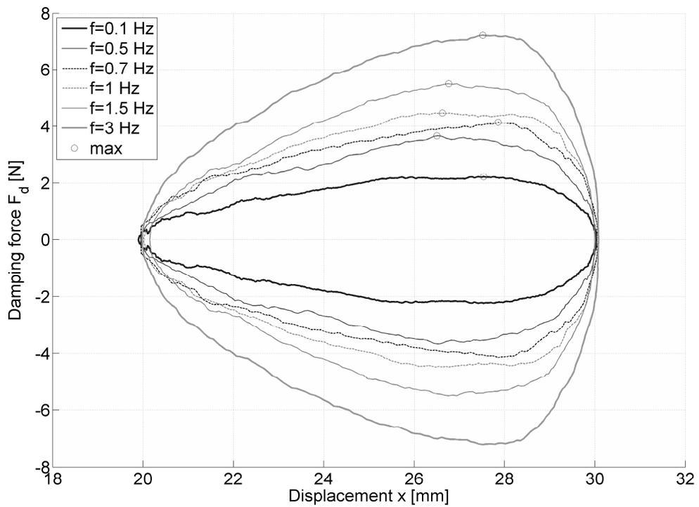
**Figure 4:** Damping force response
