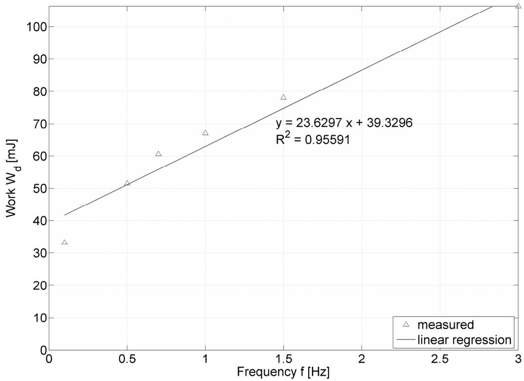
**Figure 5:** Dependence of work of damping force  $W_d$  on exciting frequency  $f$
