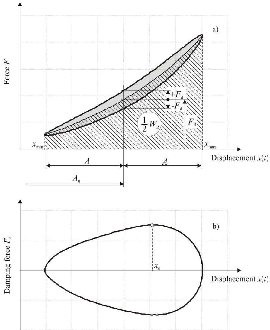
**Figure 1:** Measured force response and its decomposition
