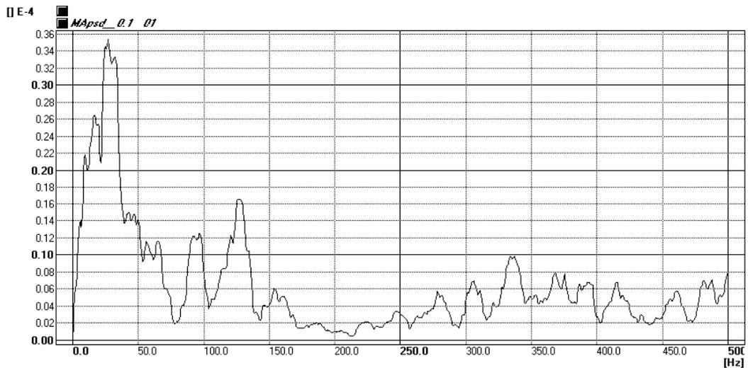
**Figure 11:** Average spectra  $S_{ws}(f)$  of the vertical sleeper acceleration  $\ddot{w}_s(t)$
