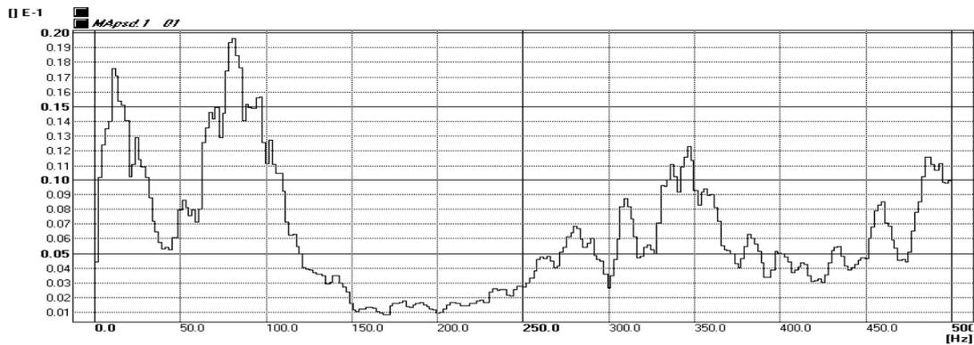
**Figure 7:** Averaged spectrum  $S_{wS}(f)$  of the vertical sleeper acceleration  $\ddot{w}_S(t)$
