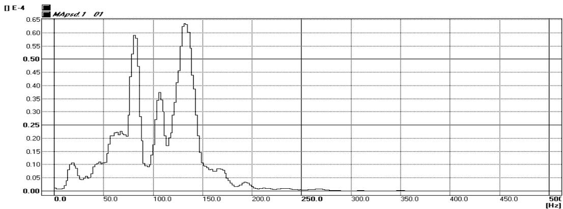
**Figure 8:** Average spectra  $S_{wB}(f)$  of the vertical ballast acceleration  $\ddot{w}_B(t)$
