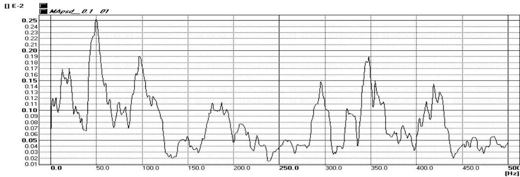
**Figure 6:** Averaged spectrum  $S_{wR}(f)$  of the vertical rail acceleration  $\ddot{w}_R(t)$
