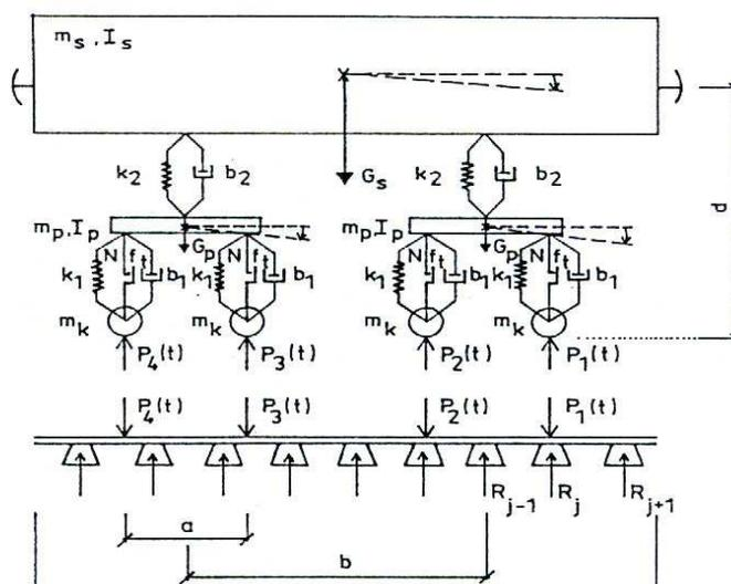
**Figure 1:** Mathematical model for dynamic interaction between moving vehicle and the track
