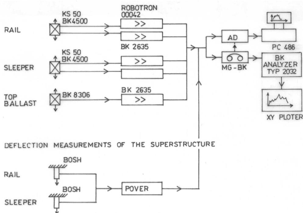
**Figure 3:** Scheme of the measurement set-up and positioning transducers in the track
