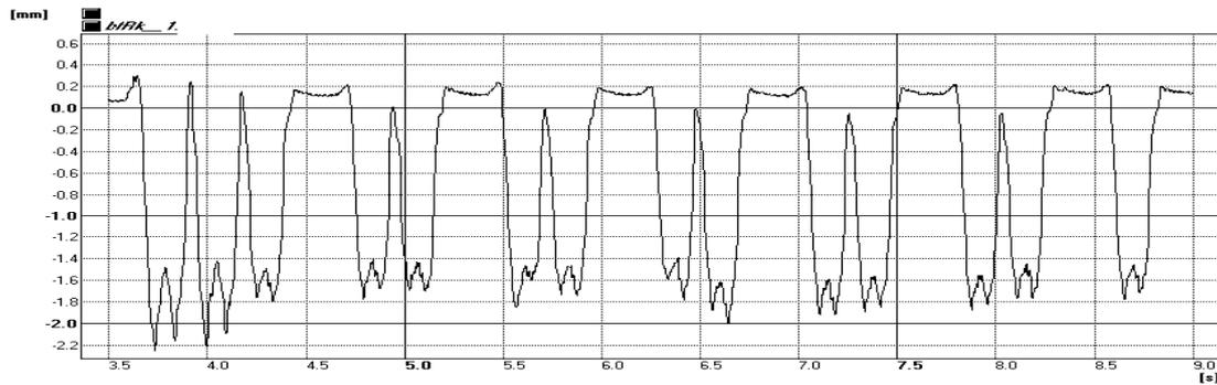
**Figure 4:** The time history of the vertical displacement of the rail for the passenger train passage L 350 + 6 coaches,  $c=115$  km/h. The sampling frequency  $f_s=1000$  Hz.
