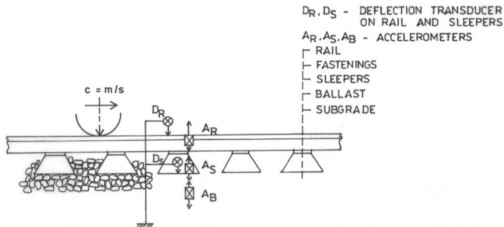
**Figure 2:** The scheme for the vehicle-track interaction measurement in the track
