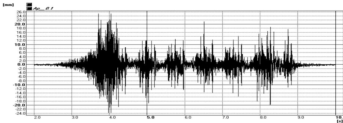
**Figure 5:** The time history of the vertical acceleration of the rail  $\ddot{w}_R(t)$
