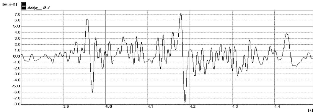
**Figure 10:** The corresponding time history of the vertical acceleration of the sleeper  $\ddot{w}_s(t)$
