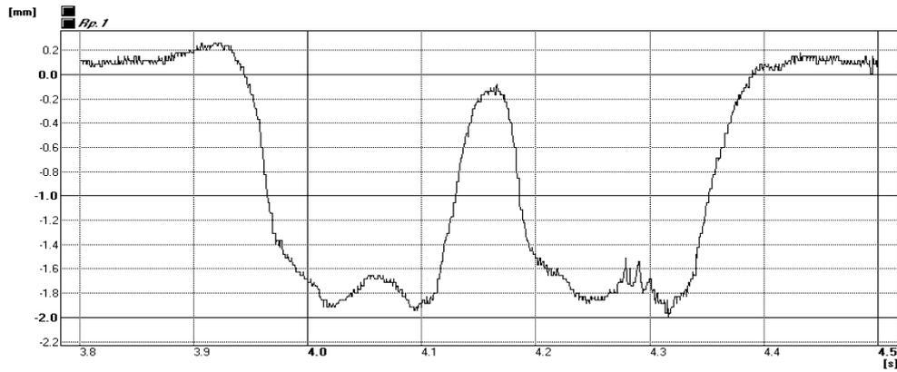
**Figure 9:** The time history of the vertical displacement of the sleeper head for the two bogies of the coaches No. 3 and 4 of the passenger train,  $c=115$  km/h,  $f_s=1000$  Hz.
