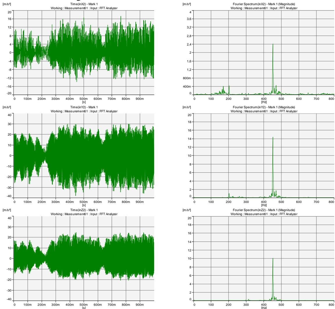
**Figure 3:** Time and frequency dependencies of acceleration for maximal vibration (1100 rpm).
