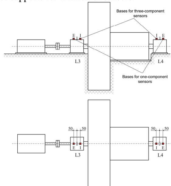
**Figure 1:** Scheme of supports positioning for fixation of sensors on bearing houses of fan.
