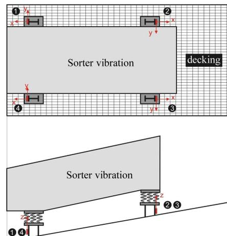
**Figure 6:** Sensors of acceleration applied on steel structure.
