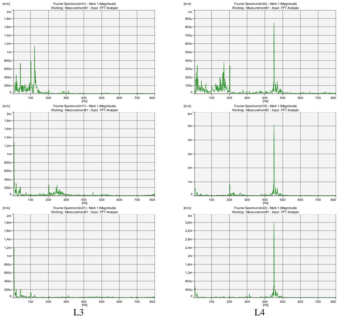
**Figure 4:** Frequency dependencies of velocity for 1100 rpm.
