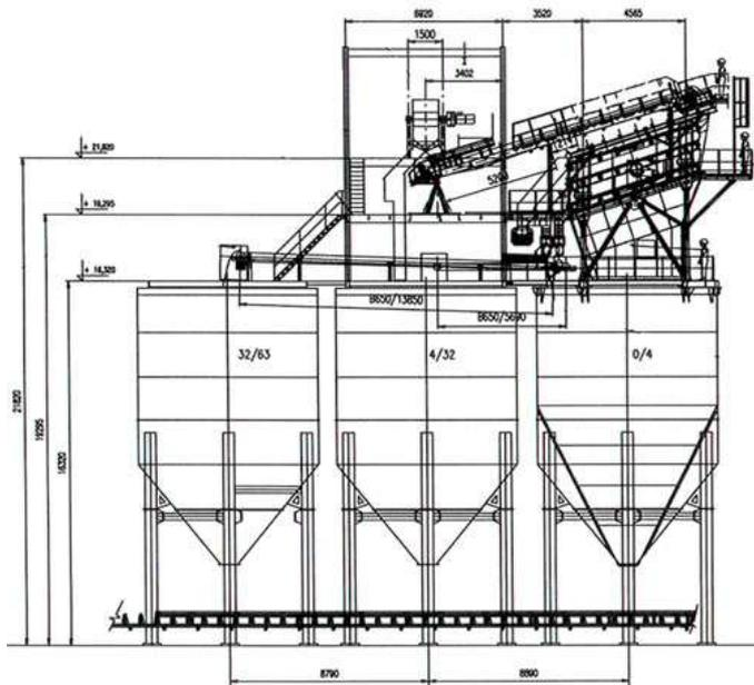
**Figure 5:** Positioning of sorter on carrying structure.
