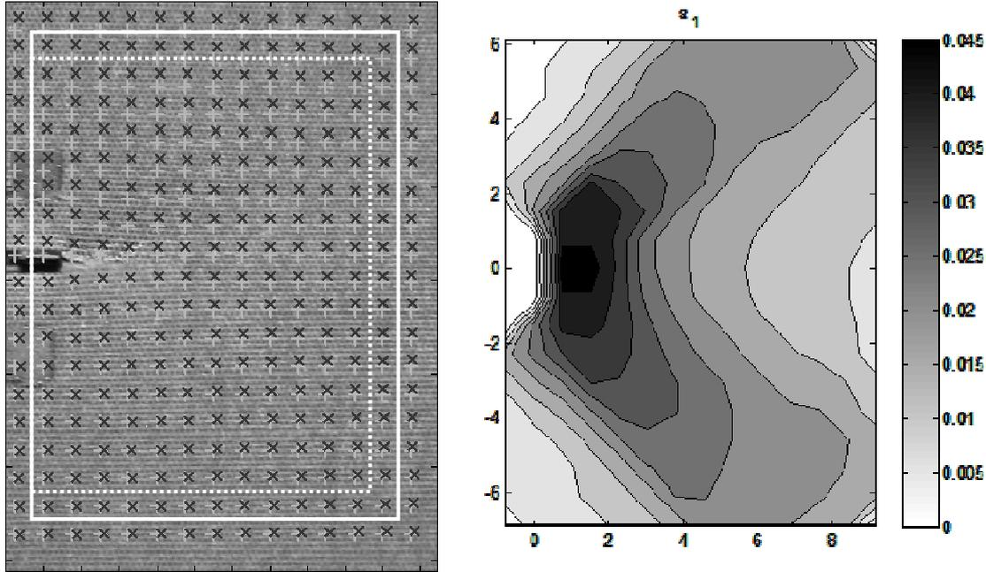
**Figure 1:** Specimen surface with DIC grid      **Figure 2:** First principal strain  $\epsilon_1$ .
