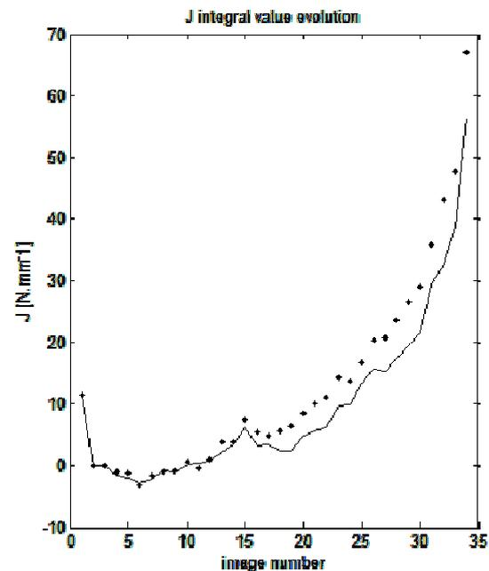
**Figure 6:** Comparison of two  $J$  integrals calculated through different paths. Integration was done on the boundary for full line, dotted line depict path one grid point closer to the crack tip.
