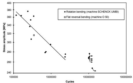
**Fig. 3.** Comparison of the flat bending fatigue test with rotating bending tests.
