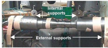
Fig. 7. Static measurement of surface strains.
