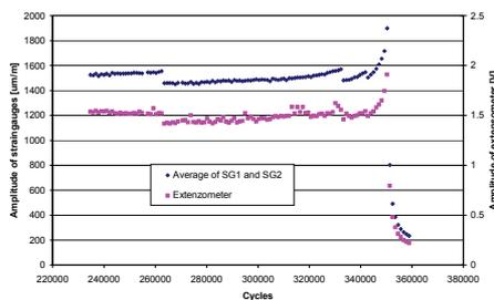
**Fig. 2.** Record of strain gauges and extensometer during fatigue test.
