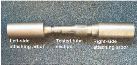
Fig. 6. Specimen with attaching arbors.
