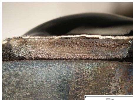
**Fig. 3.** Fracture surface with gradual fatigue crack propagation.
