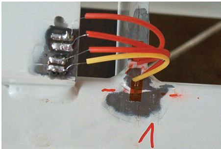
**Fig. 6.** Position of strain gauges 1 and 2.
