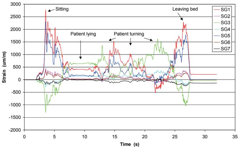
Fig. 9. Dynamic strain measurement record.
