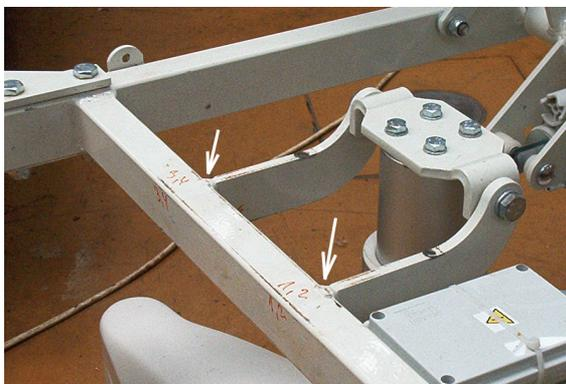
**Fig. 1.** Sickbed frame with welds between cross girder and plates, the critical welds being indicated by arrows (compression zones).
