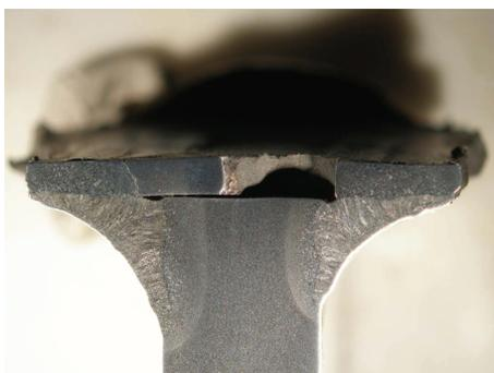
**Fig. 2.** Macro view of perpendicular cut of weld.
