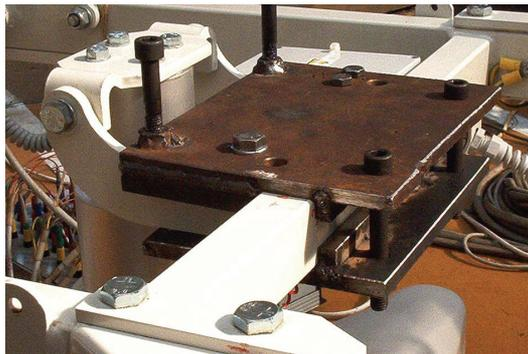
**Fig. 10.** Strengthening prototype grips with pre-stressing screws.
