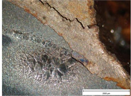
**Fig. 5.** Coarse melted structure with technological crack at zone boundary.
