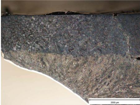
**Fig. 4.** Crack in profile wall at heat affected zone margin.
