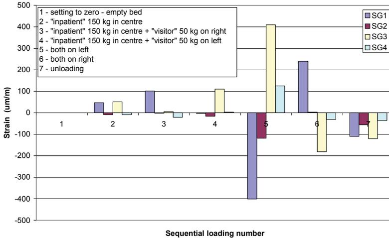
Fig. 11. Strain measurement after application of strengthening grips.
