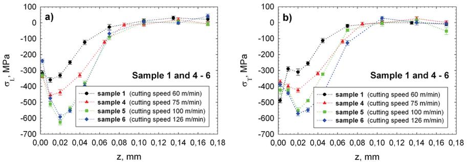
Fig. 6. Depth distribution of residual stresses  $\sigma_L$  (a) and  $\sigma_T$  (b) obtained for samples 1, 4, 5, and 6.
