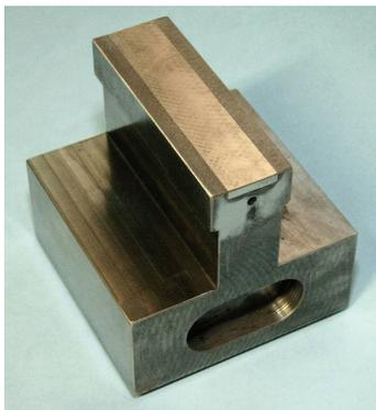
Fig. 1. Segment of a machine guide gib.
