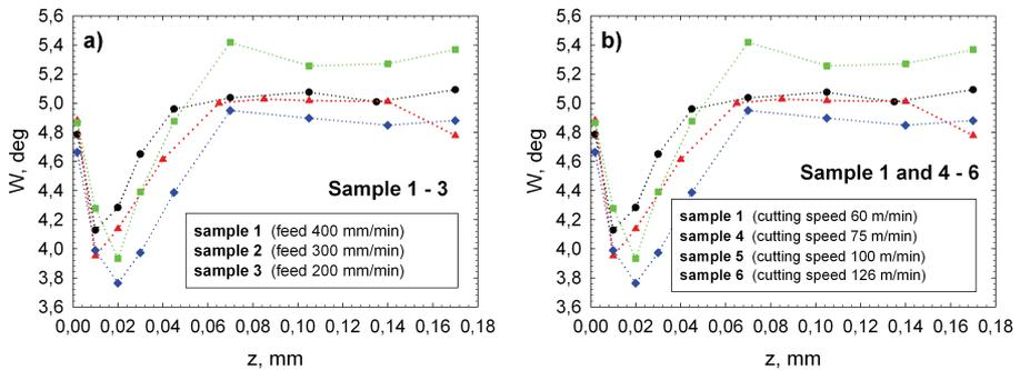
Fig. 7. Average width of the  $\{211\}$  diffraction line obtained for samples 1, 2, and 3 (a) and samples 1, 4, 5, and 6 (b).
