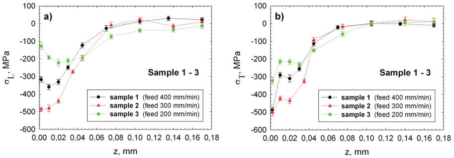
Fig. 5. Depth distribution of residual stresses  $\sigma_L$  (a) and  $\sigma_T$  (b) obtained for samples 1, 2, and 3.
