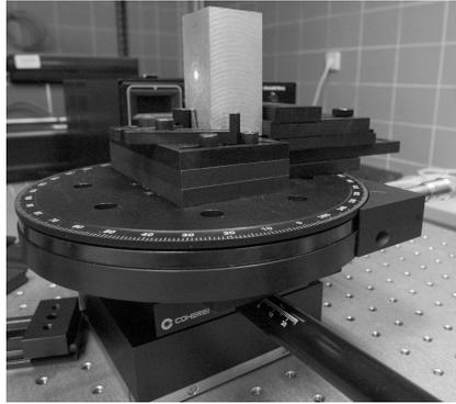
**Fig. 4.** A detailed view of an object under investigation placed on a special apparatus, which consist of translation and rotation stages.
