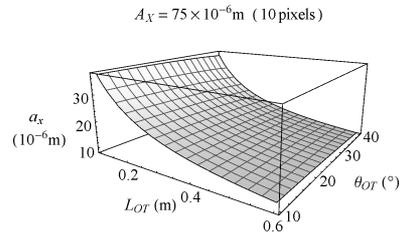
**Fig. 3.** Theoretical measurement sensitivity of in-plane object's surface translation  $a_x$  for the arrangement in Fig. 1.
