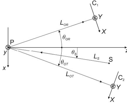
**Fig. 1.** Geometrical arrangement of the sensor for measurement of in-plane translation and rotation of object's surface.
