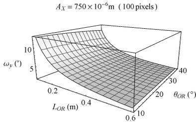
**Fig. 2.** Theoretical measurement sensitivity of in-plane object's surface rotation  $\omega_y$  for the arrangement in Fig. 1.
