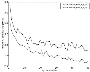
**Fig. 3.** The example of results of cyclic loading for front specimens (F). Young's moduli of elasticity decreased with increasing number of cycles. K4 – fresh specimens. K5 – frozen specimens.
