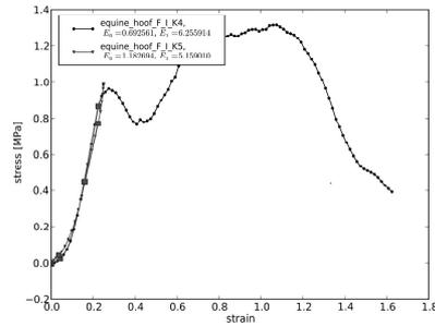
**Fig. 4.** The example of results of linearly growing loading up to rupture for front specimens (F).  $E_{\text{toe}}$  and  $E_{\text{linear}}$  - Young's moduli for toe and linear regions of elasticity, respectively. K4 – fresh specimens. K5 – frozen specimens.
