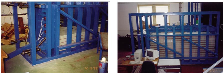
**Fig. 1.** The first stage of the experimental equipment: **a)** (Left) Preparation of the experiment E1 in 1998 with a sandy mass of the front half of an experimental space. Four red bi-component pressure sensors in the front wall are obvious, The first (upper) sensor is not placed. **b)** (Right) The equipment and the mass before the experiment E3 in 2001. The sandy mass fulfils the all experimental space into the equipment.
