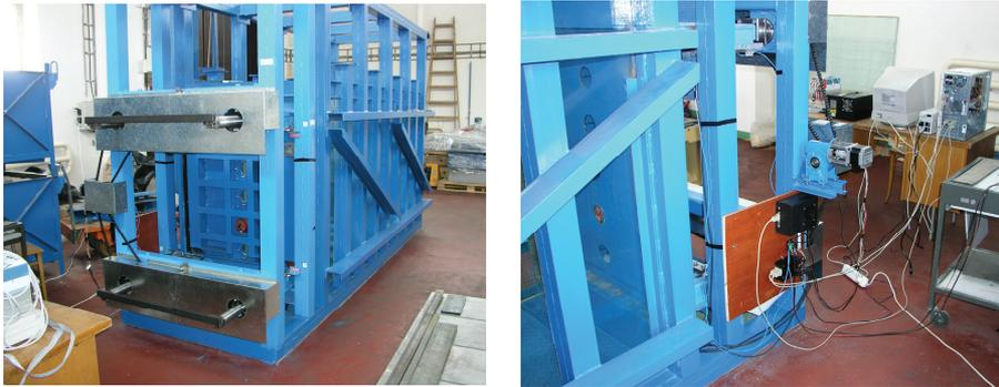
**Fig. 2. a)** (Left) Overall view of the computer-controlled front wall motor drive after the first development part and restructure of the moved front wall. The motor is on the left; the linear incremental position pick-ups near the skids cannot be seen. **b)** (Right) Motor drive in detail with hardware and computer behind.
