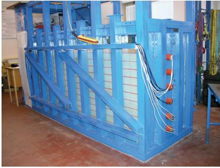
**Fig. 4.** Views of the solid back wall with six pressure sensors placed in and with the sample into.
