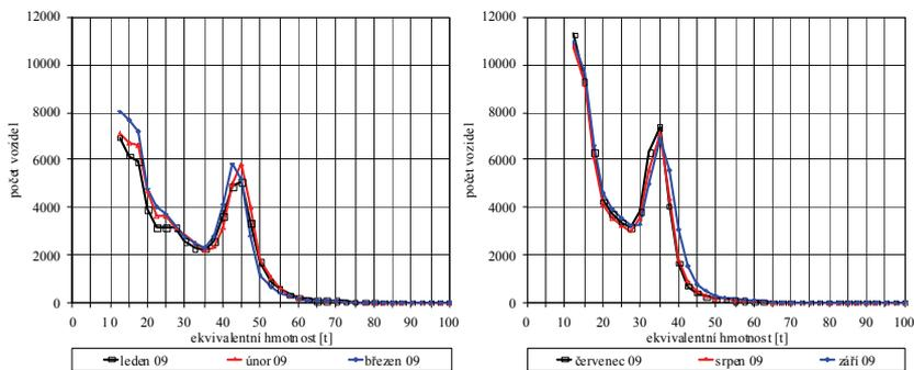
**Fig. 5.** Frequency diagrams of the number of vehicles on the bridge in Doksany classified according to the equivalent weight and monthly in the 1st and 3rd quarter of 2009.
