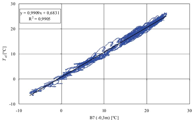
**Fig. 2.** Effective temperature  $T_{ef}$  as a function of temperature in place B7 (-0.3 m under the surface of the girder).
