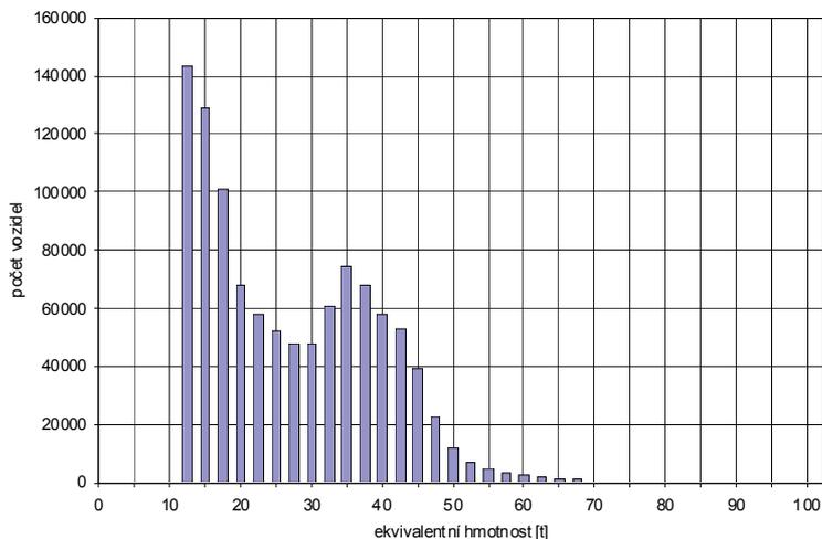
**Fig. 4.** The frequency diagram of the total number of vehicles during the period from 6 October 2008 to 31 December 2009 on the bridge in Doksany classified according to the equivalent weight.
