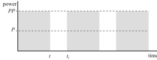
Fig. 1. Scheme of laser pulses generation.
