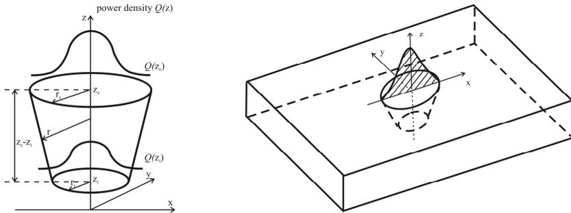
Fig. 2. Gaussian heat source applied to the material.
