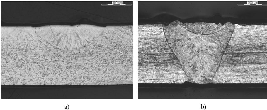
**Fig. 3.** Typical overlap pulsed laser weld cross sections a) conduction mode (4.4 J), b) penetration mode (5.9 J).
