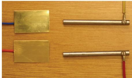
Fig. 1. Type of electrodes sunk into concrete.
