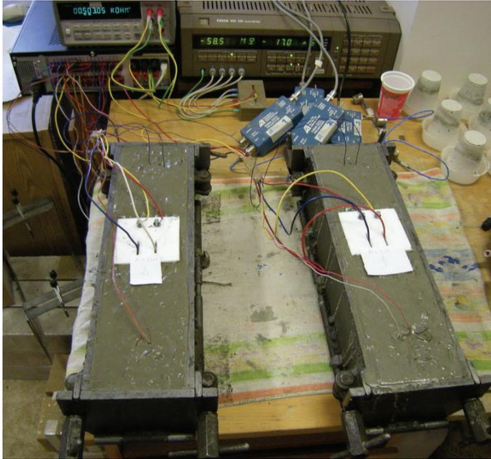
**Fig. 2.** Display of work place (concrete samples, devices and embedded electrodes). Sample No. 1 is labeled on the right, left sample is labeled number 2 during the experiment wrapped in shrink foil.
