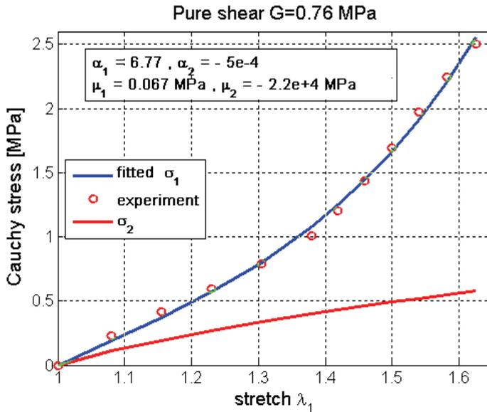
**Fig. 6.** Comparison of experimental and fitted values of the loading stress  $\sigma_1$  and the graph of the stress in transversal direction  $\sigma_2$  calculated from Eqs. (10<sub>2</sub>).
