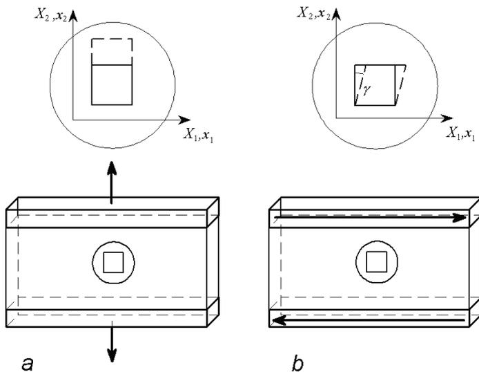
Fig. 2. Kinematics of pure shear (a) and simple shear (b).
