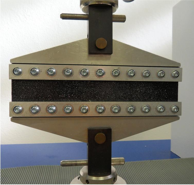
**Fig. 1.** Pure shear test device.
