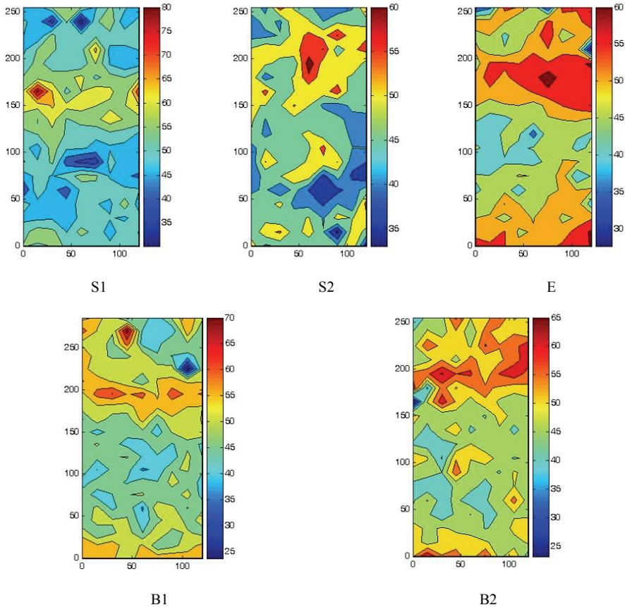
**Fig. 5.** Maps of elastic moduli on particular eggshell sections (axial coordinates are shown in  $\mu\text{m}$ , color scale of  $E$ -moduli is in GPa).
