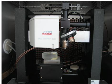
Fig. 2. Nanoindenter Nanohardness tester (CSM, Switzerland).
