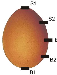
Fig. 1. Tested cross sections on the eggshell.
