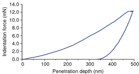
Fig. 3. Typical loading diagram received from the nanoindentation test (force vs. depth).
