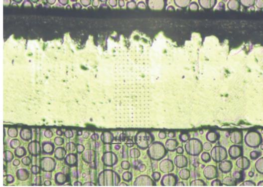
**Fig. 4.** Typical position of the indentation grid at the eggshell's cross-section (sample E).
