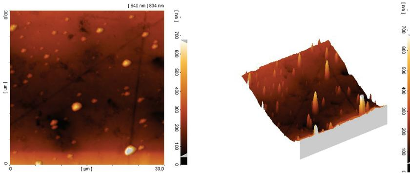
**Fig. 4.** Sample F as scanned with AFM (2D and 3D image) at 20% r.h. in time E.
