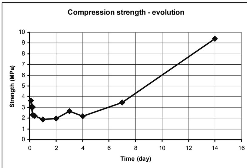
**Fig. 2.** Evolution of compression strength of gypsum.
