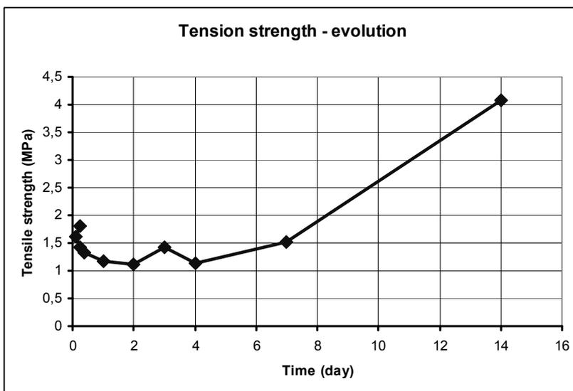
Fig. 3. Evolution of tensile strength of gypsum.
