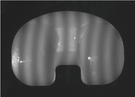
Fig. 7. Polyethylene knee insert of total knee arthroplasty.
