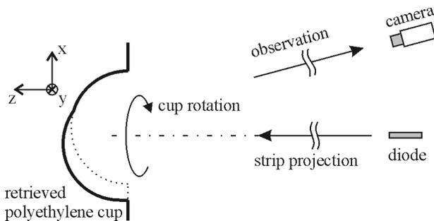
Fig. 2. Principle of the scanning profilometry.
