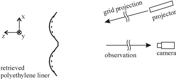
Fig. 8. Experimental setup of PSP.
