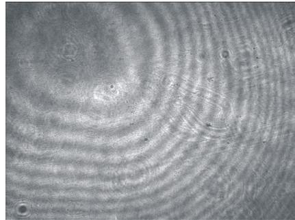
Fig. 12. Interference pattern created by sphereinterferometer.
