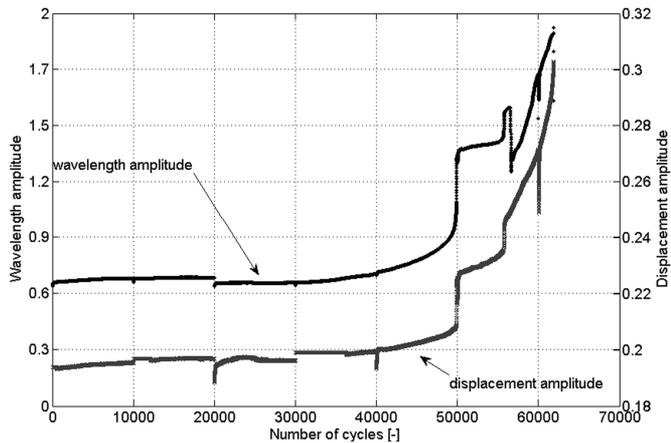
**Fig. 2.** Wavelength and displacement amplitude during the lifetime of the specimen No 1.
