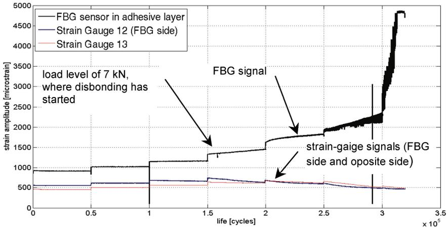
Fig. 4. (a) Example of fatigue life (Specimen SS-03).
