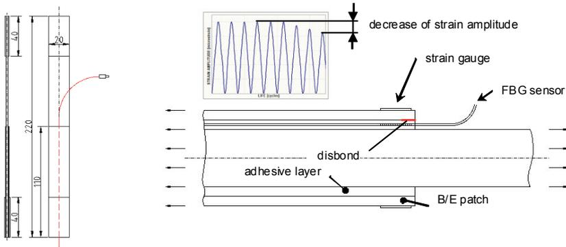
**Fig. 3.** (a) Skin Doubler Specimen (FBG sensor is marked by red line). (b) Principle of detection of disbonding during tensile fatigue loading of Skin Double Specimen.
