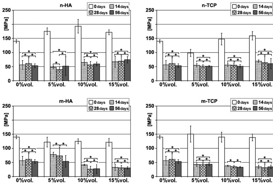
Fig. 2. The ultimate strength in bending of the composites before and after soaking in SBF (\* denotes values without statistically significant differences)
