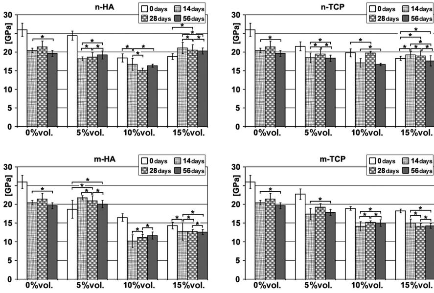
Fig. 1. Modulus of elasticity in bending of the composites before and after soaking in SBF (\* denotes values without statistically significant differences)
