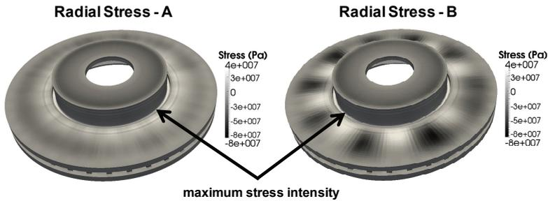
**Fig. 4.** Examples of brake disc stress fields (radial stress) obtained by FEM thermo-elastic analysis - uniform temperature (A) and hot-spots structure (B).
