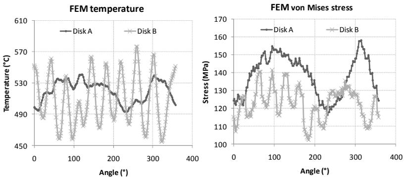
**Fig. 5.** Path graphs of the temperature and Von Mises stress in circumferential direction at the centre of the braking surface.
