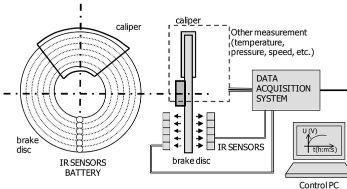
**Fig. 1.** Schematic arrangement of the measuring system for the temperature measurement on disc brakes.
