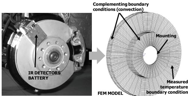
Fig. 2. Installation of the measuring system on the test car and the finite element model.
