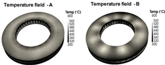
**Fig. 3.** Examples of brake disc temperature fields obtained by FEM thermal analysis - uniform temperature (A) and hot-spots structure (B).
