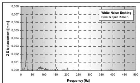
**Fig. 4b.** Frequency dependency of deviations measured by system Brüel & Kjær Pulse6 excited by white noise.
