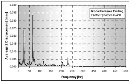
**Fig. 5a.** Frequency dependency of deviations measured by system Q-450 Dantec Dynamics excited by modal hammer.
