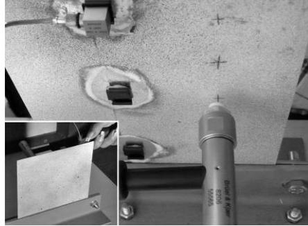
**Fig. 3b.** Excitation of specimen mechanically – modal hammer.
