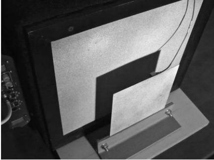
**Fig. 3a.** Excitation of specimen by acoustically acting white noise.
