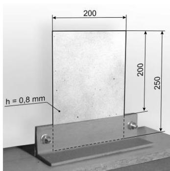
Fig. 2. Positioning of specimen and its dimensions.
