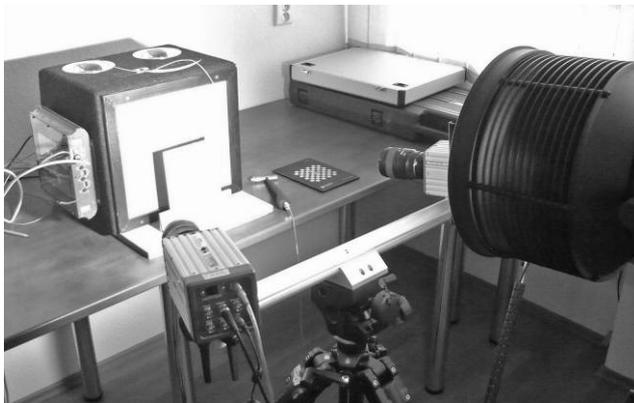
**Fig. 1.** Experimental determination of speciman modal parameters by system Q-450.
