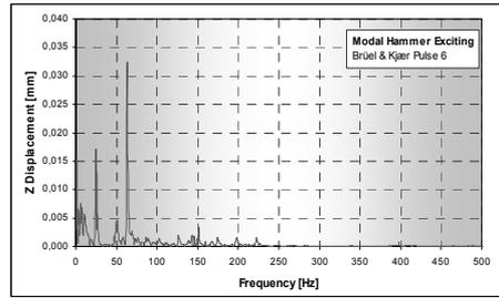
**Fig. 5b.** Frequency dependency of deviations measured by system Brüel & Kjær Pulse 6 excited by modal hammer.
