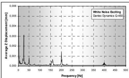
**Fig. 4a.** Frequency dependency of deviations measured by system Q-450 Dantec Dynamics excited by white noise.
