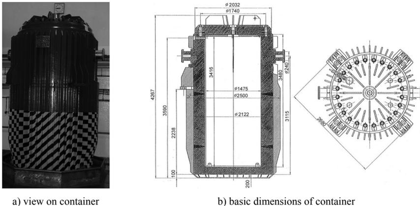
Fig. 1. Container for transportation of spent radioactive fuel.
