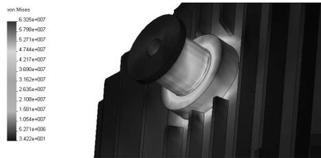
**Fig. 4.** The field of equivalent stresses in a journal of container during its lifting by crane with the hooks fastened on journals
