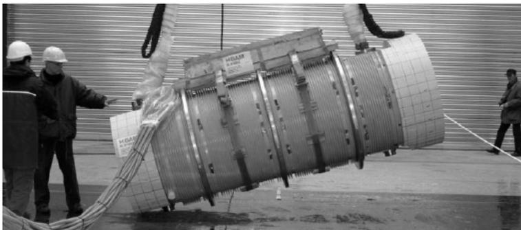
**Fig. 8.** Container with impact shock limiter [6].
