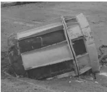
**Fig. 5.** Container after landing on concrete block from high 200 m [7].
