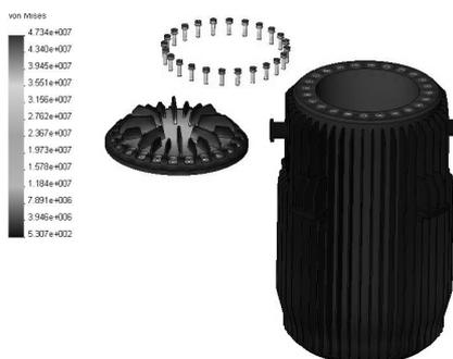
**Fig. 3.** The field of equivalent stresses in container with internal pressure 740 kPa.
