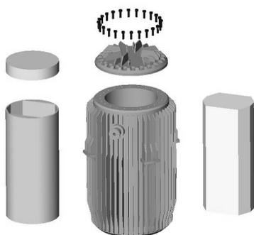
**Fig. 2.** Model of individual parts of container for computation by FEM.
