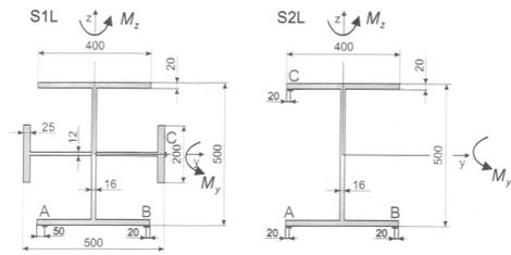
**Fig. 7.** Locations of strain-gages for hole drilling method.
