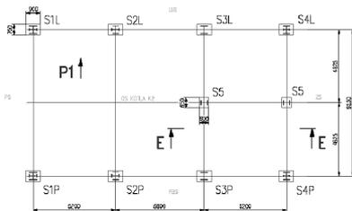
**Fig. 6.** Labeling of column of supporting structure and approximate locations of strain-gage application.
