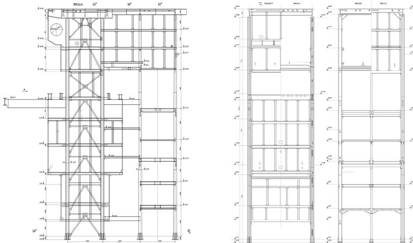
Fig. 1. Original boiler supporting structure.
