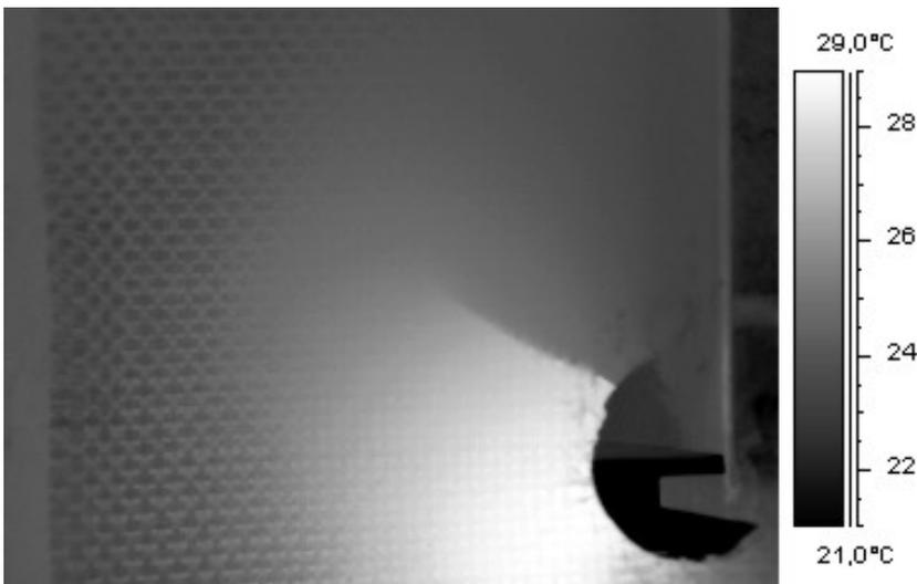
**Fig. 4.** Thermograph of the surface temperature around the opening. The crack acts as a barrier against the heat flow and therefore a notable discontinuity the temperature field develops.
