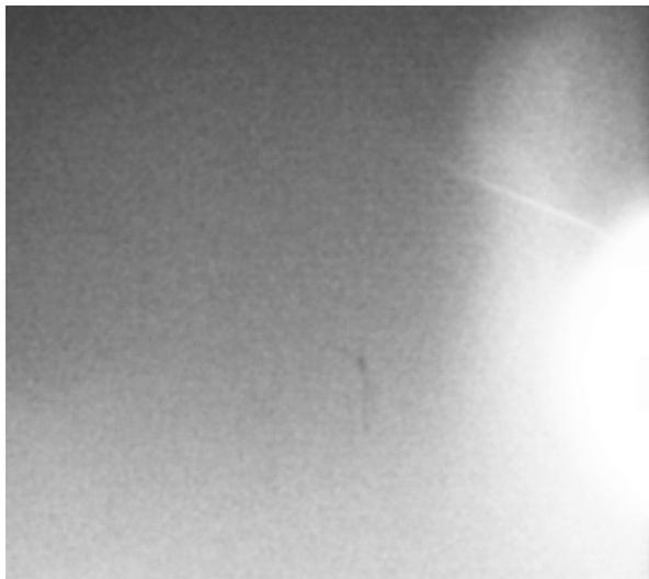
**Fig. 2.** The radiograph of elements' opening (round white area on the right side of the image) with a fatigue crack depicted as a thin bright line propagating from the opening towards upper left corner of the image.
