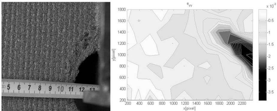
**Fig. 3.** The left part of the figure depicts two color paint sprayed on carbon fibre patch with attached measuring tape. The opening is shown as a black circular hole. On the right side of the figure strains determined by DIC method are presented in contour plots. The area of the highest strains corresponding to the darkest shadows of gray indicates the location and the extent of the crack.
