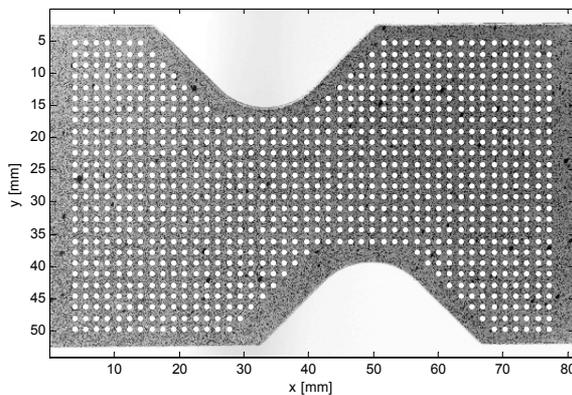
**Fig. 2.** The view of the evaluated part of the specimen surface with reference orthogonal grid.
