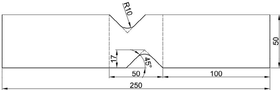
**Fig. 1.** Draft of a flat EN 10 204 Al-alloy specimen with asymmetric notches. Length units given in mm.
