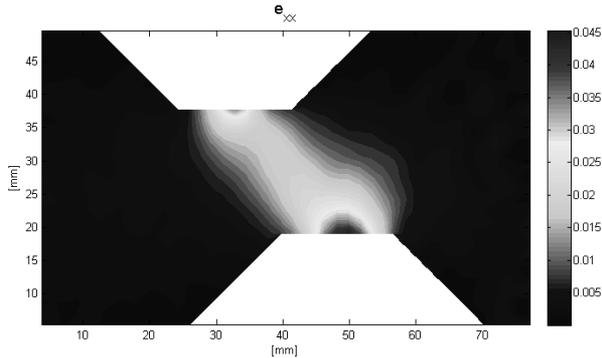
Fig. 3. Strain field  $\epsilon_{xx}$  calculated by the DIC software.
