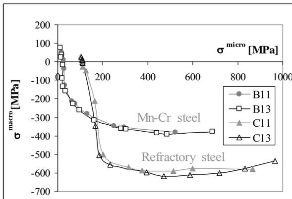
**Fig. 3.** Parametric plot of macrostresses vs. microstresses for materials *B* and *C*
