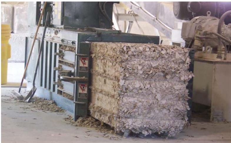
**Fig. 2.** The line for pressing waste paper. Taken from <http://www.drywallrecycle.com>
