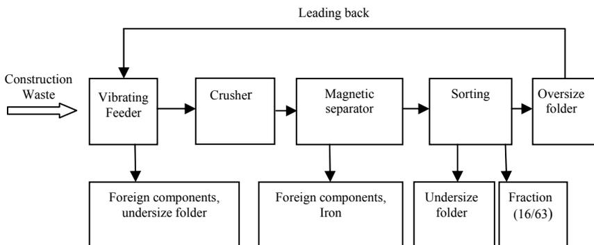
**Fig. 3.** Diagram of the combined recycling line for waste plaster
