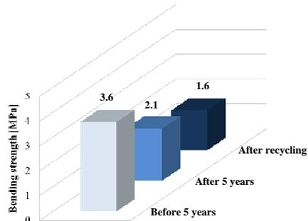
**Fig. 6.** Bending strengths of tested gypsum samples
