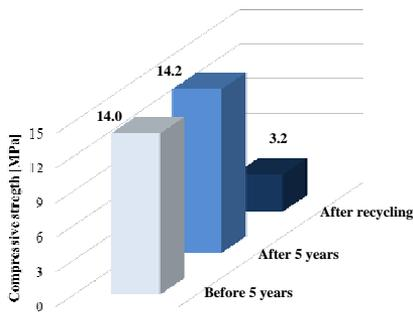
**Fig. 5.** Compressive strengths of tested gypsum samples
