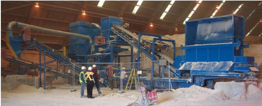
**Fig. 1.** Recycling line for waste plaster al. NWGR – UK, Adapted from <http://www.nwgyplsum.com>
